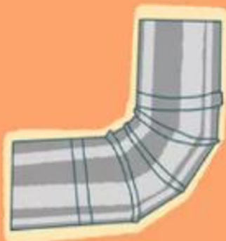
Rigid Metal Duct
